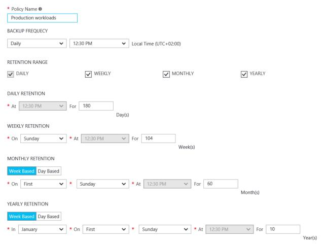
The most time-consuming operation in backup is the copying of data from the primary storage to the backup storage, and the time taken is dependent on a host of factors like network latency, available IOPS on the primary storage account, and available IOPS on the backup storage account. Azure Backup implements an optimized blob copy that ensures constant, predictable IO and backup times. Azure Backup does additional processing to determine the
