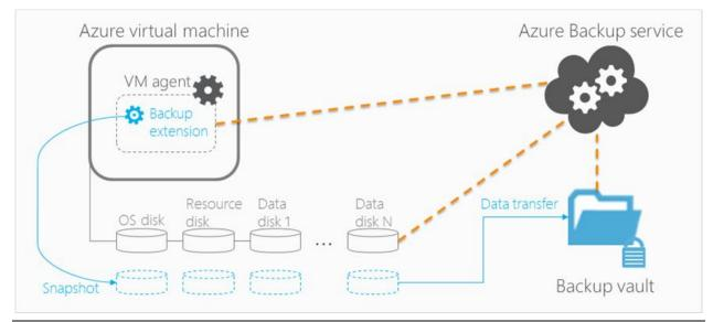
The foundation of every Azure Backup is the Recovery Services Vault. The vault could be based on Geo-Redundant Storage (GRS) or Locally-Redundant Storage (LRS). GRS provides three copies of your backup data in the primary region and three more copies in another region to be protected from regional disasters. A best practice is to use Geo-Redundant-Storage, especially for any production workloads. The storage type needs to be configured before you start protecting machines.
