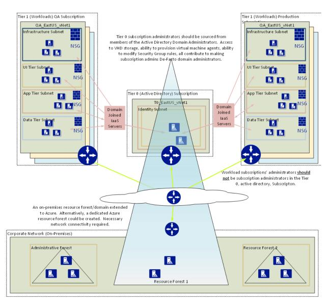
QA and production networks share the same dedicated ExpressRoute circuit to on-premises resources. They are separated into distinct subscriptions to allow separation of access and to allow the QA subscription to scale on its own without impacting production.
