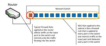
For example, if a Network Security Group is created and a Network Security Group rule is defined that denies inbound Remote Desktop Protocol (RDP) traffic for all addresses over port 3389, no virtual machine outside the subnet can connect via RDP to a virtual machine that is connected to the subnet, and no virtual machine connected to the subnet can connect via RDP to any other connected virtual machine.
