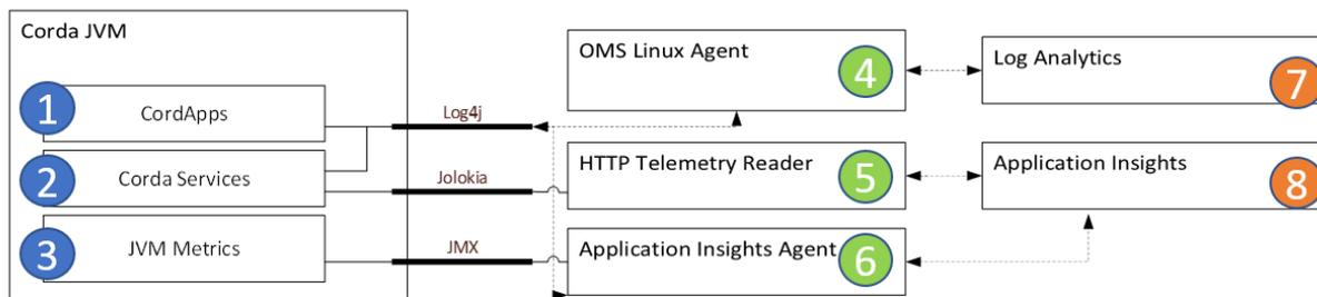
From a JVM perspective we have 3 sources of logs that can feed into different components, which we can configure to trace telemetry into either Log Analytics or Application Insights.
