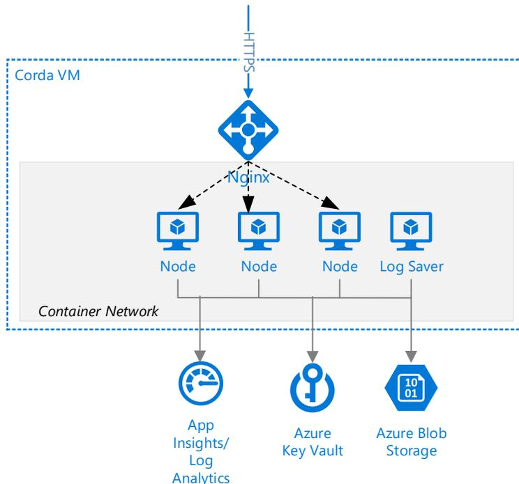
The pattern which can use to monitor the Corda node application is a *sidecar* pattern. We can achieve this by pairing the Corda node application, which can run either in an IaaS Virtual Machine instance or in a container, next to another instance where we run the “log saver agent” which will then send syslog information into Log Analytics.
