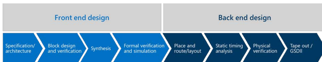
Figure 1 - Overview of Silicon Design Flow
